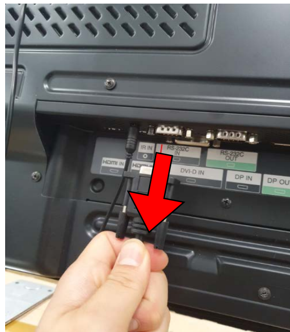
■ RS232C Cable – 1. Turn it counterclockwise. 2. After unlocking the holder, pull it out vertically.
