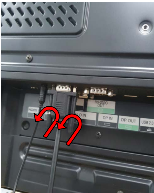
■ RS232C Cable – 1. Turn it counterclockwise. 2. After unlocking the holder, pull it out vertically.
