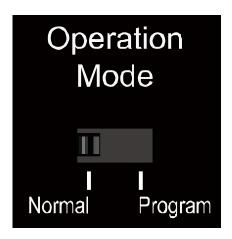
2. According to the silk prints nearby ("Program" for firmware update, "Normal" for RS232 transmission), change the switcher positions to set RS232 port's function.
