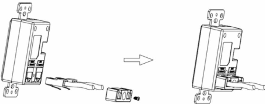
Step2: Put the HDMI Wall Plate Extender to your outlet box and fix it.
