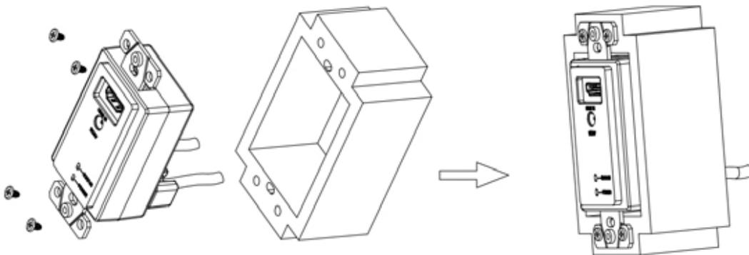
Step3: Put the wall plate to the extender and use included 6#-32x7/32" screws to fix it.
