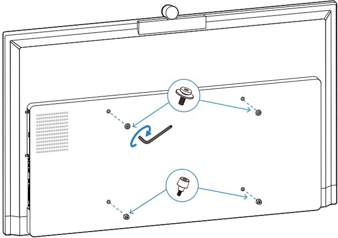
**7** Mount the display and insert the gourd-shaped mounting pegs into the corresponding installation positions on the bracket.
