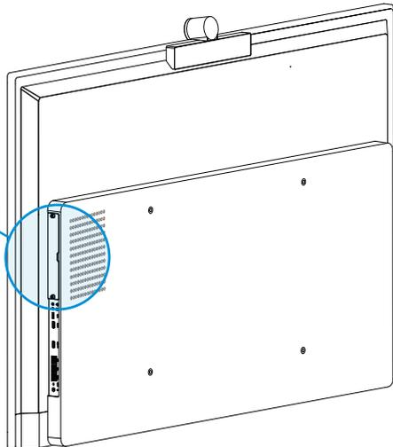
**6** Install gourd-shaped mounting pegs and supporting screws on the rear of the display, and ensure that they are tightened correctly.
