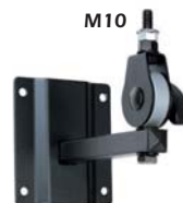
EU-01480 Adjustable wall mount - Wall plate: W105 x H120 mm - Length: 170 mm - Max load: 10 Kg / Wht: 0.8 Kg - Rotation: 0 - 360° / Tilt: 0 - 90°
