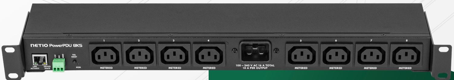
Each of eight outputs can be independently controlled from the web interface (switched on / off or power-cycled). To switch the outputs on in a sequence (after a power-up or when power is restored), a power-up delay interval can be configured for each output individually.
