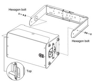
**6** Adjust the speaker angle, then tighten the bolts until the speaker is securely affixed.
