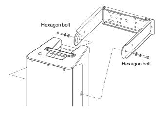
**5** Adjust the speaker angle, then tighten the bolts until the speaker is securely affixed.
