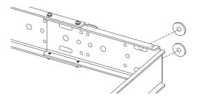
**5** Use the included M8x25 hexagon bolts, spring washers, and flat washers to attach the speaker to the U bracket.
