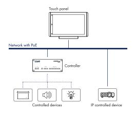
The following diagram describes the use of a touch panel with IP-controlled devices only. This configuration allows creating a cost-effective distributed control solution where the touch panel serves as a controller and graphic user interface in one box. In Cue Visual Composer touch panels and controllers are programmed in the same way, which makes it possible to use touch panels as fully functional control units.
