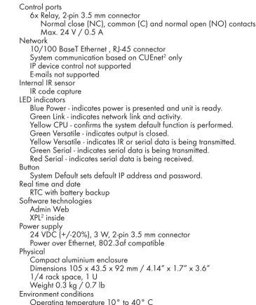
Environment conditions Operating temperature 10° to 40° C Storage temperature 0° to 60° C Relative humidity 10% to 90% non-condensing
