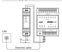
Delivered DIN rail power supply 24 VDC can be used for areas without PoE infrastructure.
