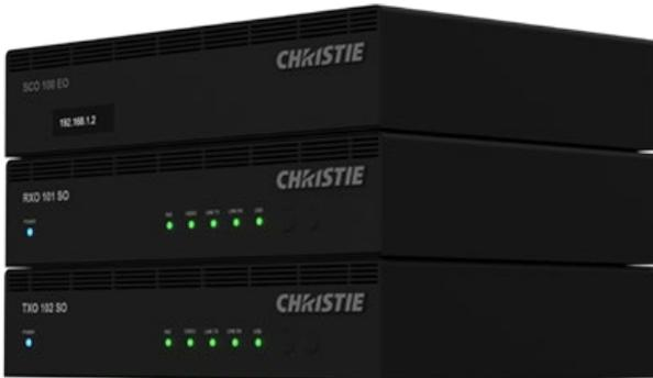
The Transmitter processes audiovisual sources and control signals to deliver uncompressed, zero-frame latency, artifact-free content over 10G networks. The Terra Transmitter supports video resolutions up to 4K@60Hz and accepts various port connections, including HDMI 2.0, USB, HDCP 2.2, DisplayPort 1.2, serial RS-232, EDID and more. This powerful and flexible device does not require additional devices to process signals.
