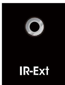
User can use the IR receiver cable to change the IR receiver position. If controlling the HDBaseT Matrix through the 1/8" (3.5 mm) input jack on the rear panel, connect the IR cable directly to the matrix rear IR receiver extension sockets.
