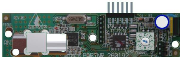
Install the receiver PCB on the 261377 in the small connector between the white PCB holders (see image).
