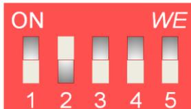
Dipswitch position 3 = Soft start/stop on/off - soft start/stop "on"
