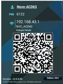
The default setting is Hotspot mode. Directly connect to the SSID broadcasted by the device.
