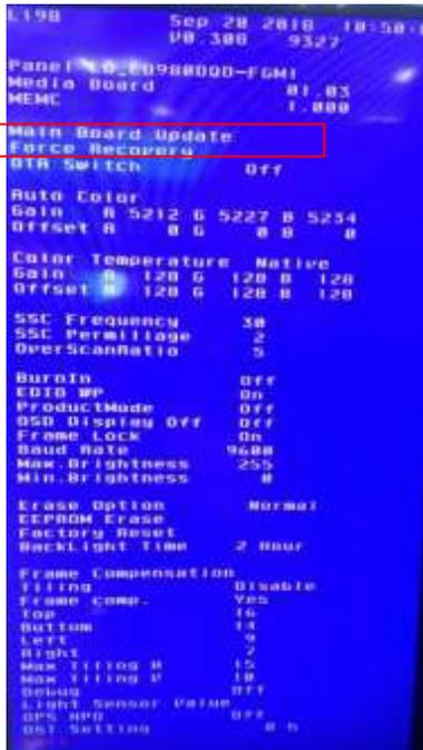
Check if firmware has been upgraded: press the home button on the RC, select configuration 2, select On the right monitor information, the firmware version must match the installed version.
