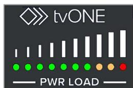
If the red LED is lit, reduce the amount of power drawn by disconnecting one or more devices, until only green and yellow LEDs are lit. If you want to run more devices, use an additional ONERack Spider PSU.
