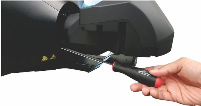
3. To remove the lens, with the screwdriver press the **Lens Release** button (shown below) and rotate the lens counterclockwise by a quarter.
