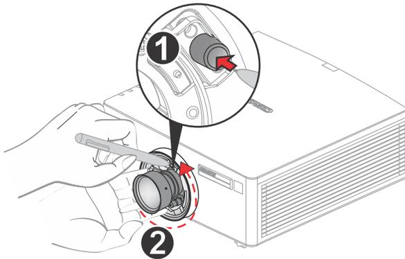
2. Remove the lens through the front of the projector.
