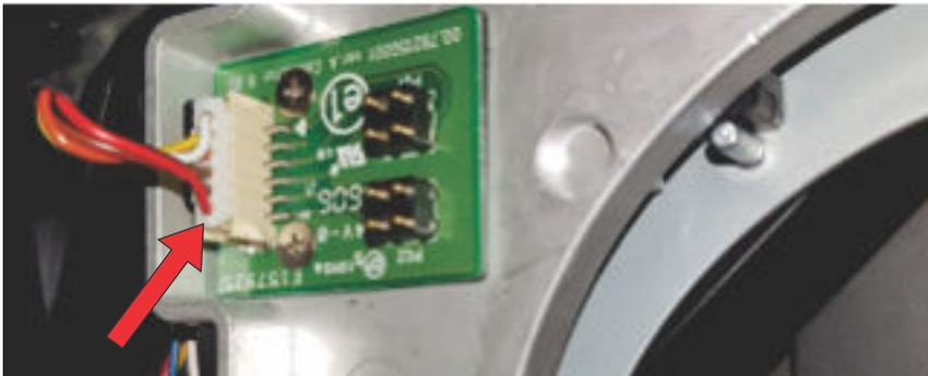
6. Insert the new ultra short throw lens boresight adapter in the projector. When inserting the new boresight adapter, ensure it does not scratch the aperture casing of the projector.
