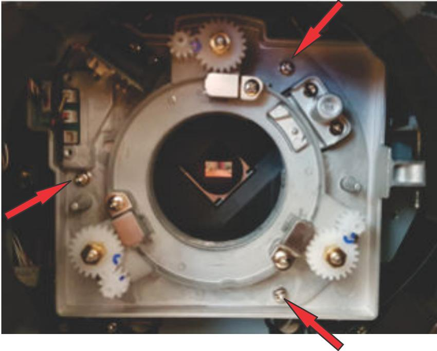
3. Rotate the standard boresight adapter and remove from the projector. When removing the boresight adapter, ensure it does not scratch the aperture casing of the projector.
