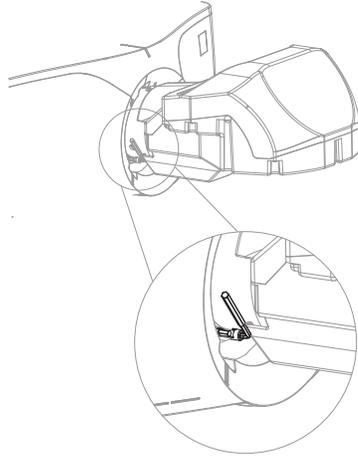
6. To adjust the boresight for optimized image quality, use the L-shaped socket key.
