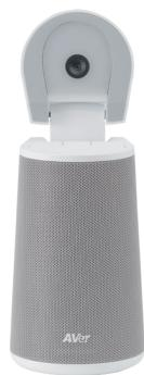
The A30 is a multifunctional and all-in-one purpose camera. It's the first in the industry to feature a visualiser, microphone, and speaker in one device. At the same time, the A30 can be utilised as a webcam for video conferencing, and a document camera to visualise materials, providing the ultimate pleasure of hybrid/mobile teaching.
