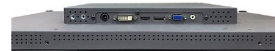
Multiple video inputs (HDMI, DVI, VGA, DisplayPort) make possible effortless system integration
