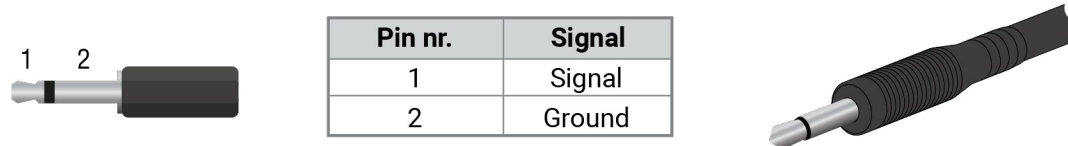
Microphone audio plug pin assignments
