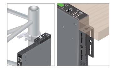
Care must be taken to ensure proper ventilation of MODEX when designing any system. Side ventilation holes must not be covered. If the ventilation of a MODEX is limited to a closed space (MODEX is built into furniture for example), the designer shall provide satisfactory ventilation of that space to prevent excessive heat build-up inside.
