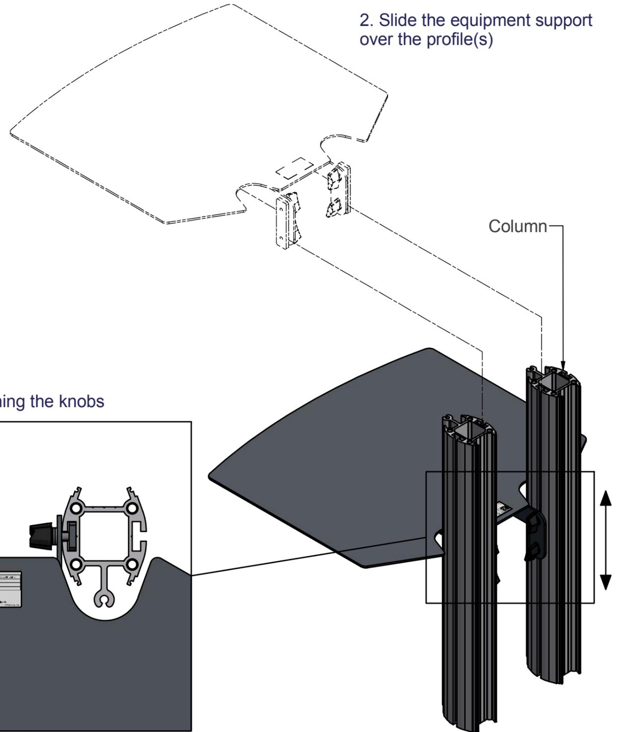
3. Adjust the height by tightening the knobs
