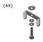
M6 Nylon Ring Clamping bracket M6 flat washer M6 spring washer M6X30 Panhead screw
