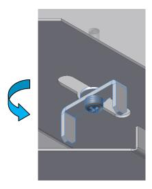
**9.** Position the inner cover plates inside the lift finishing.
