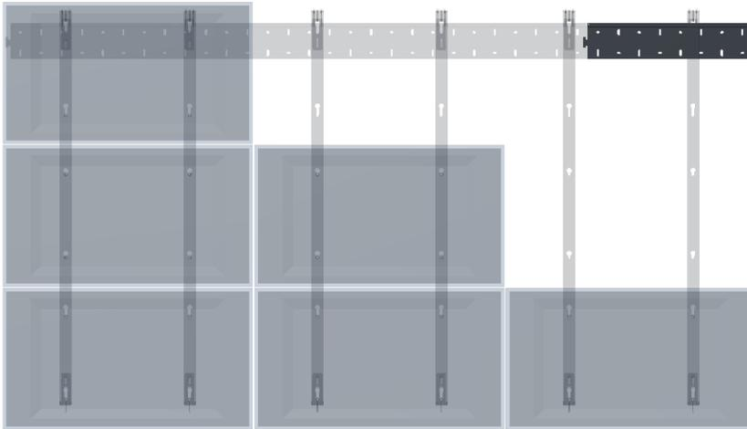
**VWM-MA-?-?**, Monitor mounting arms suitable for 1, 2 or 3 stacked monitors. The type of MA arm is determined by the diagonal and screen height.
