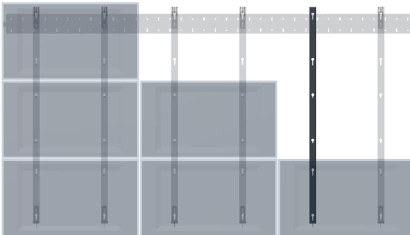
The monitors are being installed with the by Audipack provided special mounting cams. These cams can be inserted at the back of the monitors. There are several cams available with different thread dimensions.
